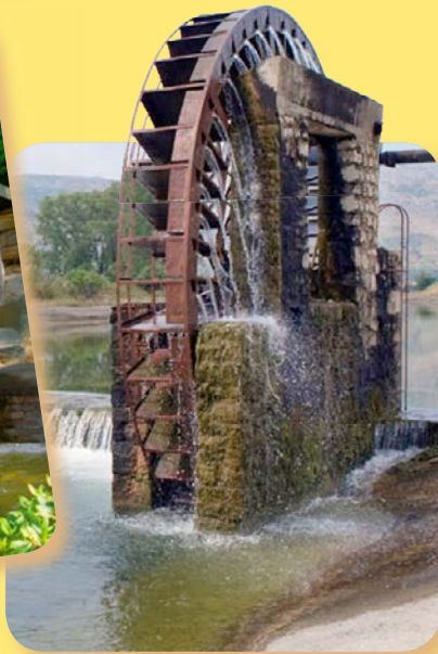
A breastshot wheel sits lower in the water. The water fills buckets from the side of the wheel.
